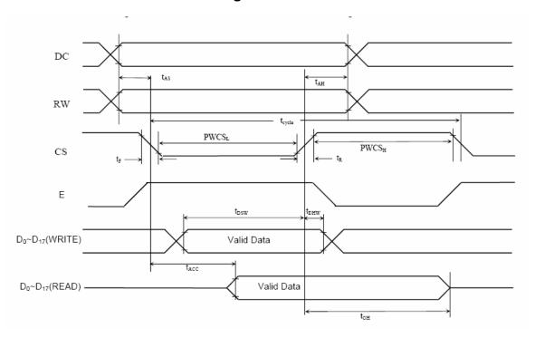
$(Ta = -20^{\circ}C \sim 70^{\circ}C \ VDDIO = 1.65 \sim 3.6V)$
