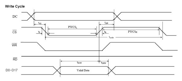
$(Ta = -20^{\circ}C \sim 70^{\circ}C \ VDDIO = 1.65 \sim 3.6V)$
